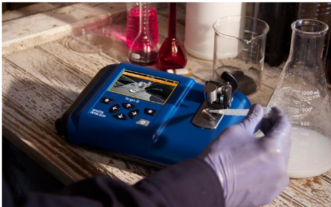
Picture 1. Sample being placed on the diamond ATR element for pressing during analysis
