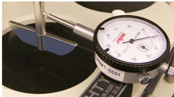
Figure 4. Dial test indicator (runout gauge) showing probe in contact with installed paddle shaft (Note that the measurement of basket wobble is similar with the probe tip in contact with the bottom basket rim). A different probe tip design may be used such as a large flat tip.
