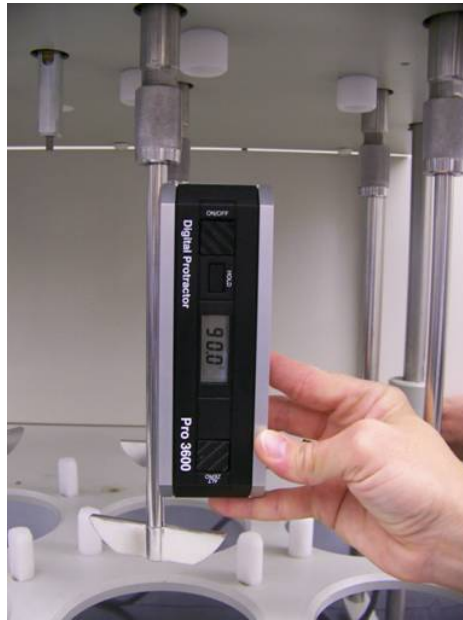
Figure 2. Measurement of the verticality of the stirring element using digital protractor.
