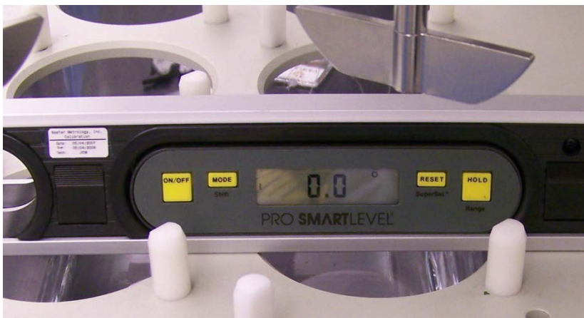
Figure 1. Electronic level giving 0.0° reading on the base plate of a test assembly.
