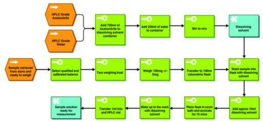
Figure 6. The sample preparation step, broken down into detailed substeps.
