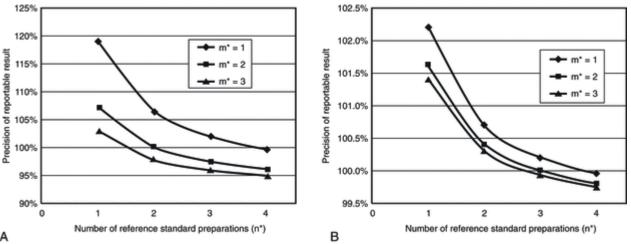
Figure 2. Dependence of intermediate precision on the format of calibration. The calculated precisions for alternative calibration formats are normalized with respect to the intermediate precision obtained in the precision study. The following relative standard deviations for the reference standard were used: API, example A:  $CV_{RR} = 0.76\%$ ,  $CV_{RP} = 0.14\%$ ,  $CV_{I} = 0.58\%$ ; Tablet, example B:  $CV_{RR} = 1.42\%$ ,  $CV_{RP} = 0.35\%$ ,  $CV_{I} = 0.22\%$ .
