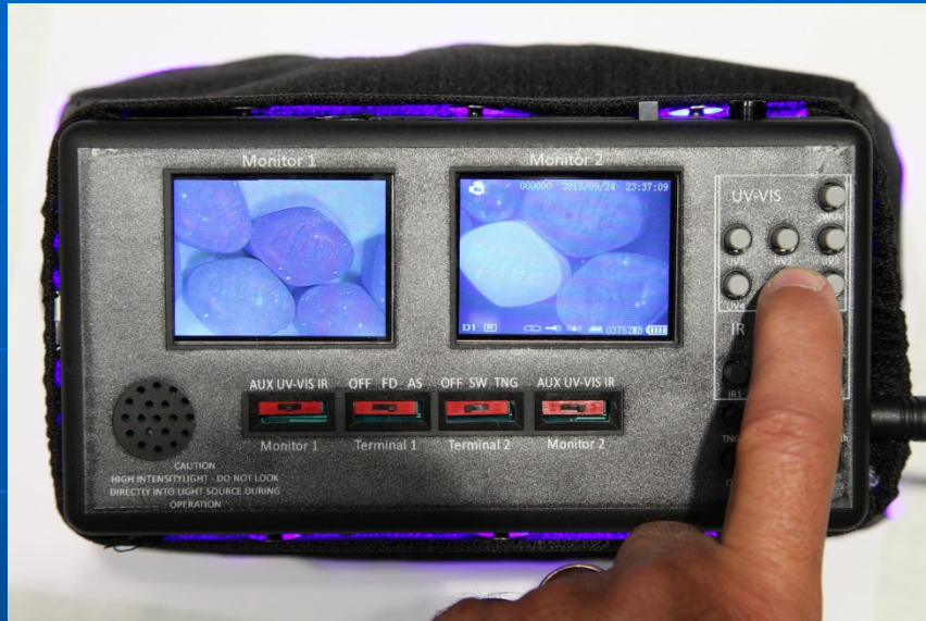
UV-VIS and IR side by side live view mode comparison
