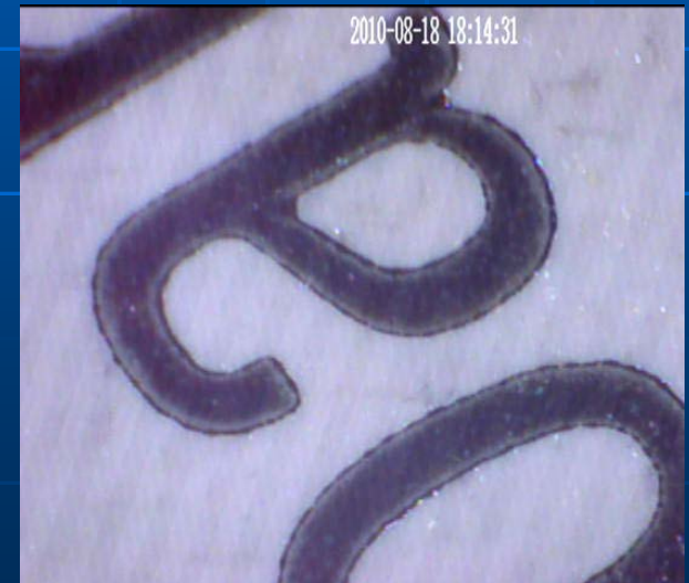
Flexographic Printing Process 100x
