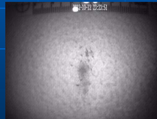
Photo 2: Dark jacket with blood stain under IR imaging 1050
