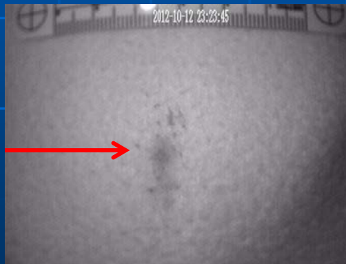
Photo 3: Dark jacket with blood stain under IR imaging 850
